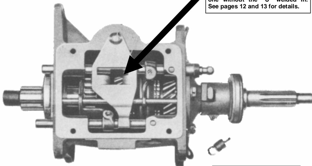
Unhook the clutch release bearing return spring.
