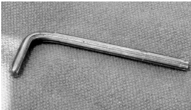
This may look somewhat like an Allen wrench but it is NOT. Basically it is a fluted wrench. These tools are available from various jeep parts dealers for approximately $5 to $10.
