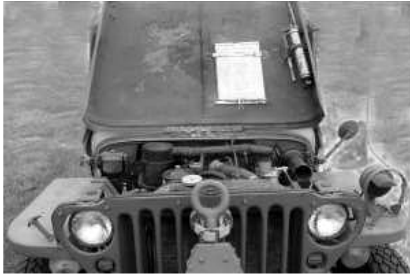
Figure 3. A view from the front before my latest rebuild. Note the Ford style lube chart holder (made from plans included in Ray Cowdery's book All American Wonder , the grease gun and holder and also, the tandem hitch. The hitch was designed to connect two jeeps together to act as a prime mover for field guns like the 105mm.
